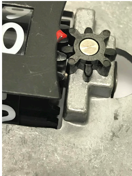
Figure 3-20: Pinion counter wheel alignment on whole numbers
